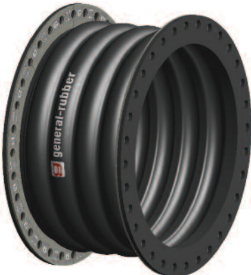
Style 1104 Quadruple (4) Wide Arch Rubber Expansion Joint with quadruple the movement and one-quarter the spring rate of style 1101. 36" ID X 24" FF shown.
