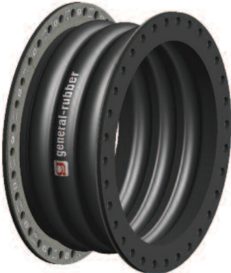
Style 1103 Triple (3) Wide Arch Rubber Expansion Joint with triple the movement and one-third the spring rate of style 1101. 36" ID X 20" FF shown.
