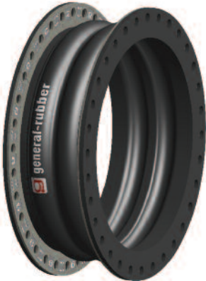
Style 1102 Double (2) Wide Arch Rubber Expansion Joint with twice the movement and half the spring rate of style 1101. 36" ID X 15" FF shown.
