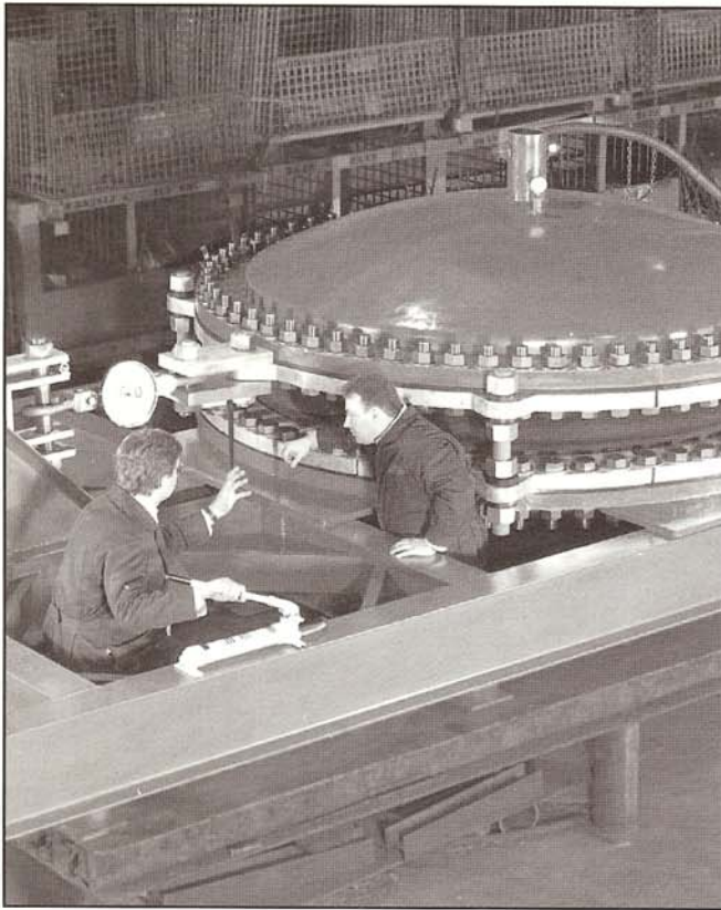
Figure 3. Expansion Joint Stiffness Testing
