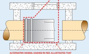
ALTERNATIVE DESIGN, DASHED IN RED, ILLUSTRATES THAT IMPROVED BOTTOM CLEARANCE IS OBTAINED WHEN TOP CLEARANCE IS SACRIFICED.
