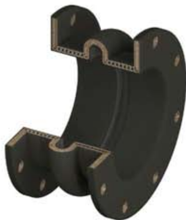
Figure 2A: Single Narrow Arch Type Expansion Joint
