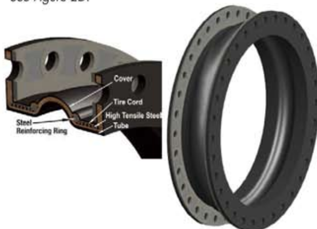
Figure 2D: Molded Wide Arch Metallic Reinforced Type Expansion Joint
