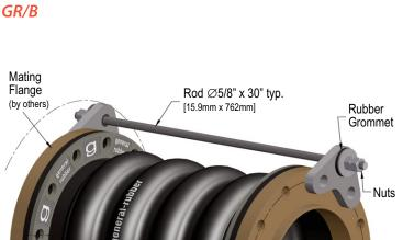
8" ID x 18" F/F (DN150mm x 457mm) - 150-lb Drilling | 1104-0008-3.16
