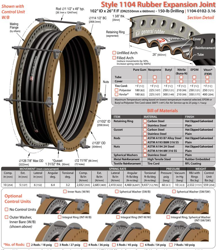
\*Gusset thickness and pressure listed above are for carbon steel gussets and ASTM A193 B7 rods. Contact General Rubber for stainless steel pressures and thicknesses. Contact General Rubber Corporation for full product specifications, Warnings and installation instructions.
