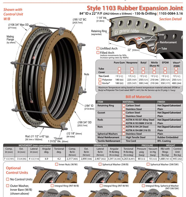
\*Gusset thickness and pressure listed above are for carbon steel gussets and ASTM A193 B7 rods. Contact General Rubber for stainless steel pressures and thicknesses. Contact General Rubber Corporation for full product specifications, Warnings and installation instructions.
