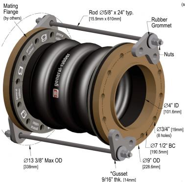
4" ID x 14" F/F (DN100mm x 356mm) - 150-lb Drilling | 1103-0004-3.16
