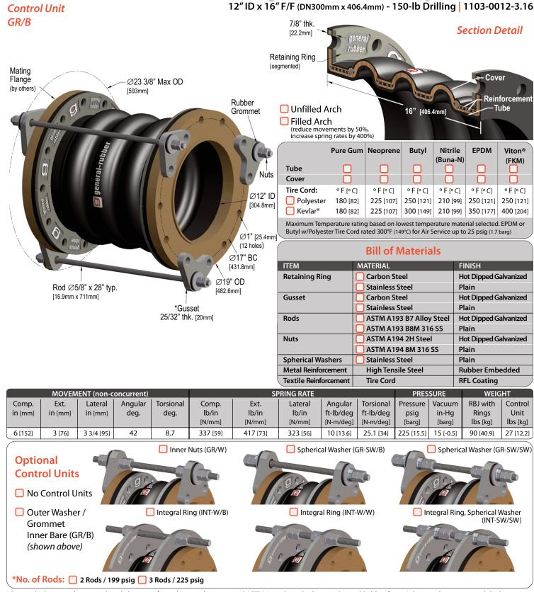
\*Gusset thickness and pressure listed above are for carbon steel gussets and ASTM A193 B7 rods. Contact General Rubber for stainless steel pressures and thicknesses. Contact General Rubber Corporation for full product specifications, Warnings and installation instructions.
