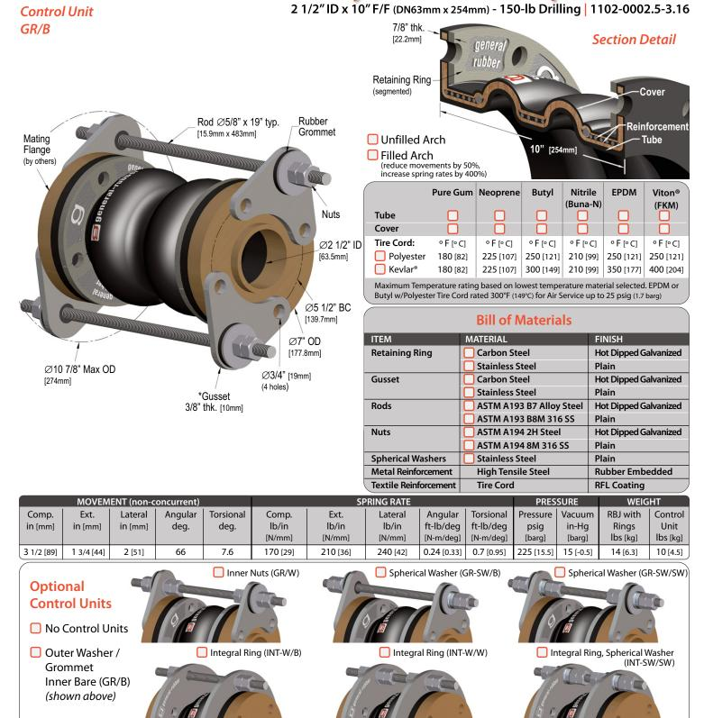
\*Gusset thickness and pressure listed above are for carbon steel gussets and ASTM A193 B7 rods. Contact General Rubber for stainless steel pressures and thicknesses. Contact General Rubber Corporation for full product specifications, Warnings and installation instructions.
