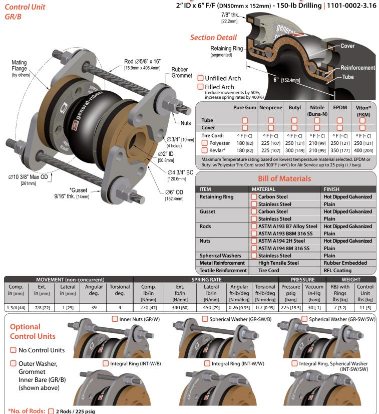
\*Gusset thickness and pressure listed above are for carbon steel gussets and ASTM A193 B7 rods. Contact General Rubber for stainless steel pressures and thicknesses. Contact General Rubber Corporation for full product specifications, Warnings and installation instructions. © 2016 General Rubber Corporation, All Rights Reserved
