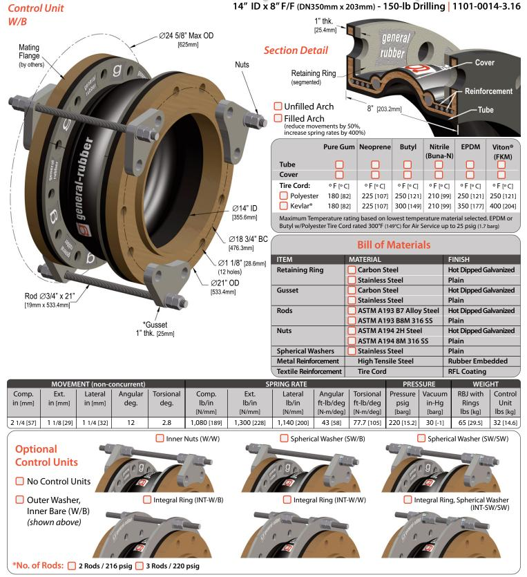
\*Gusset thickness and pressures listed above are for carbon steel gussets and ASTM A193 B7 rods. Contact General Rubber for stainless steel pressures and thicknesses. Contact General Rubber Corporation for full product specifications, Warnings and installation instructions.
