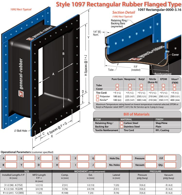
Available in hot dipped galvanized rings/bars, custom offsets as well as reducing arrangements. Available in external or internal flanges. Extension movement capabilities can be increased with additional pre-compression during installation.
